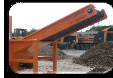
Figure 1.8: Density Separator Module
