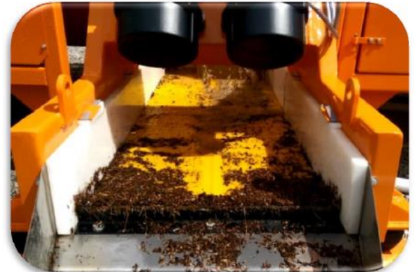
Figure 1.4 Vibrating Screen with Perforations
