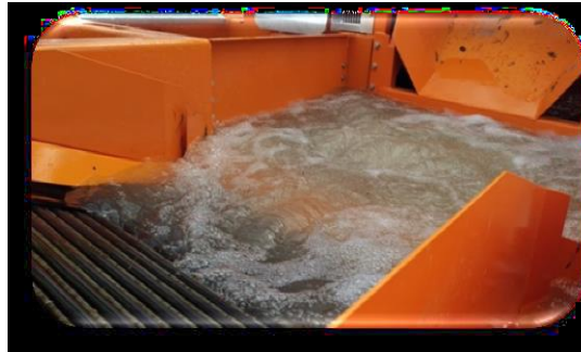
Figure 1.6: Density Separator Module
