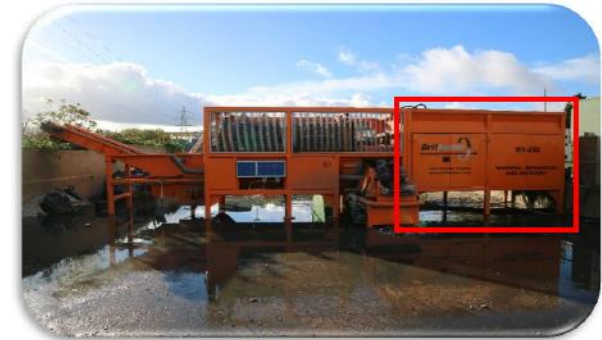
Figure 1.1 Feed Hopper Section
