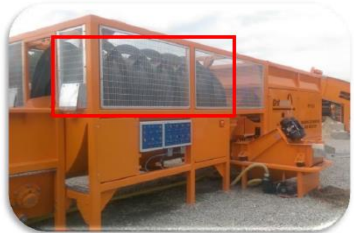
Figure 1.2 Trommel Drum Section
