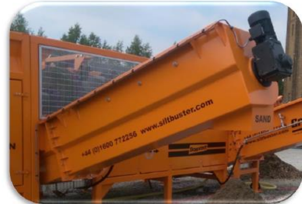
Figure 1.3 Coarse Sand Auger
